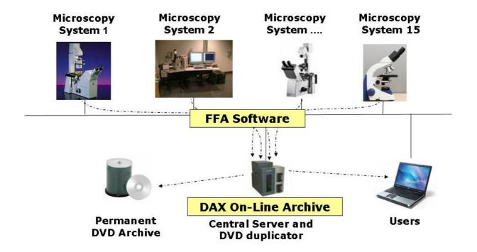
The data on the **central server** is archived fully automatically to DVD. This involves a **robotic mechanism that burns and labels all archive disks automatically**.
