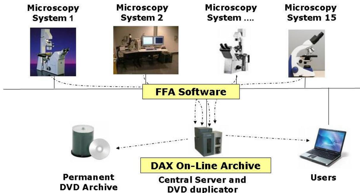
The data on the **central server** is archived fully automatically to DVD. This involves a **robotic mechanism that burns and labels all archive disks automatically.**
